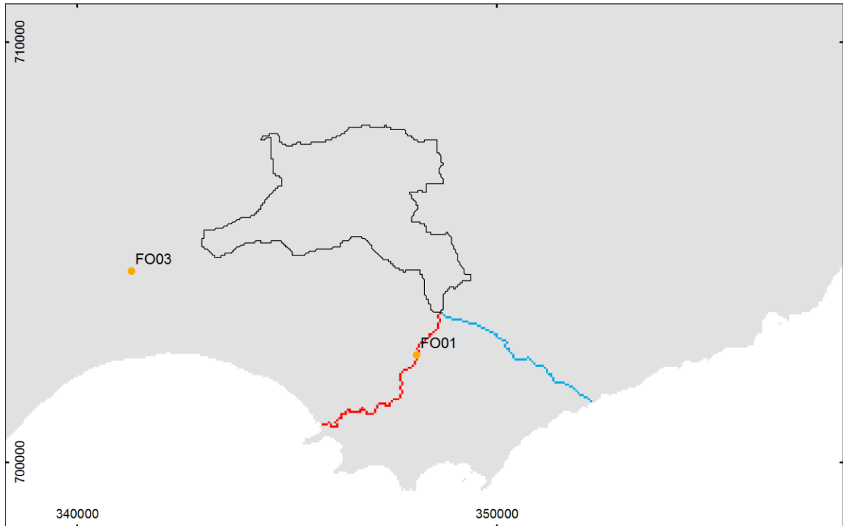
Figure 55 Illustration of changes to introduce corrections suggested by SEPA near Inverie Burn which seemed to have the highest impact on the calibration sites. The original catchment area (black outline) was 12.75 sq km. Red cells are cells where cumulative catchment area of the new raster was higher than what the original IHD TM suggested, blue cells are cells where cumulative catchment area of the new raster was lower than the original IHD TM suggested. Orange points are RICT calibration sites labelled with RICT_ID.
