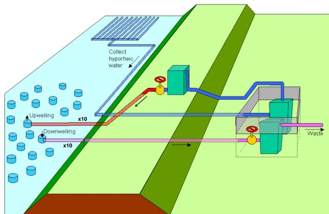
Fig 1. Schematic diagram of experimental structure showing directions of water movement
