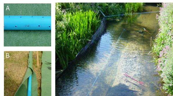
Fig 4. a) 20,000 hyporheic water collection holes; b) wrapping collection pipes in capillary matting; c) one of ten 30cm deep x10m length streambed trenches for hyporheic water collection pipes
